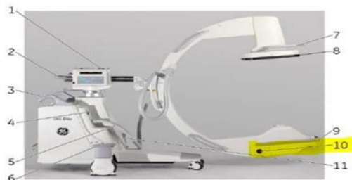
Figure 3-39: Common C-Arm component identification (Super C-Arm pictured)
